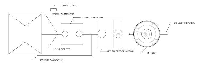
Figure 11—Plan View Showing Grease Trap
