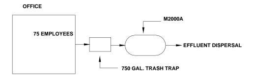
Figure 10—Commercial Occupancy Nayadic Installation with Flow Equalization
