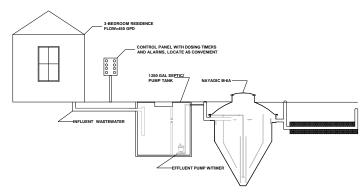
Figure 9 - Navadic Installation With Flow Equalization
